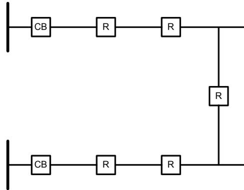
Fig. 5. Basic looped distribution feeder without communications
