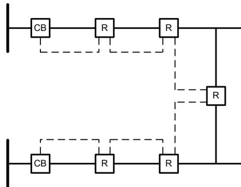
Fig. 6. Basic looped distribution feeder with peer-to-peer communications
