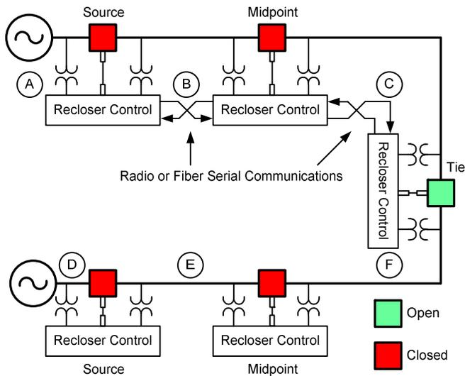
Fig. 1. Distributed control for protection and ANR
