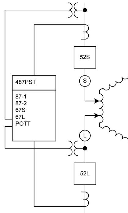
Fig. 8. Single-line diagram of PST protection system
