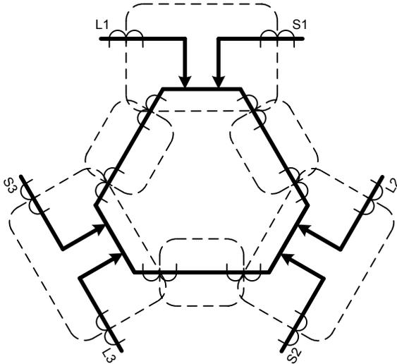
Fig. 4. Differential protection for single-core PST, 87P
