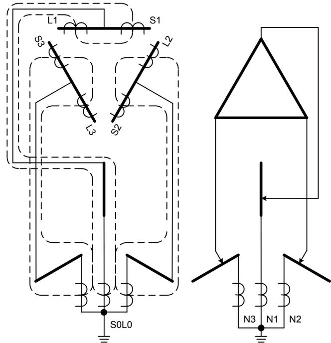
Fig. 5. Primary differential protection for two-core PST, 87P
