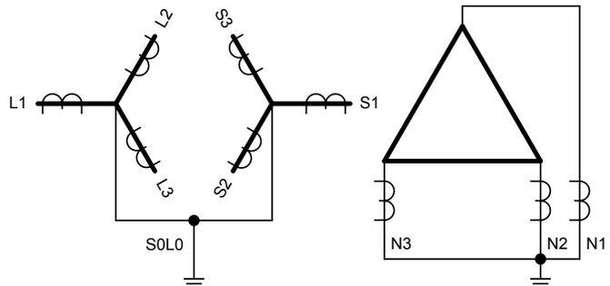
Fig. 6. Secondary differential protection for two-core PST, 87S
