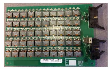
Fig. 18. Transmission line model section used to simulate a 3.8-mile singlephase segment. The thyristor-based fault model is visible at the lower righthand side. The complete line model uses 10 sections.
