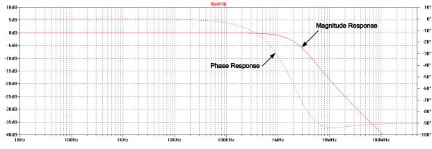
Fig. 7. Frequency response of the relay analog circuitry (excluding anti-aliasing filter).
