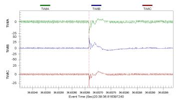
Fig. 28. Phase currents at Drummond for the B-phase-to-ground fault at 38.16 miles from the Goshen terminal.
