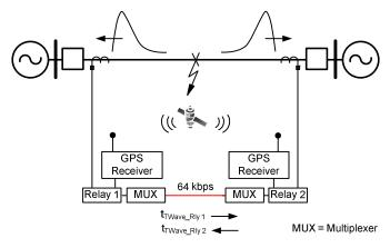
Fig. 4. Relays exchange the time of arrival of the TW to estimate the fault location in real time.
