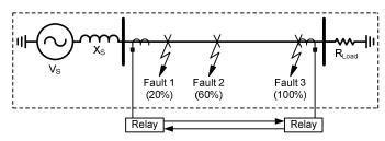
Fig. 17. Physical transmission line model.
