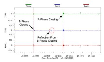
Fig. 23. TW phase currents captured during line energization.
