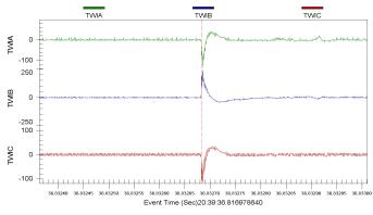
Fig. 27. Phase currents at Goshen for the B-phase-to-ground fault at 38.16 miles from the Goshen terminal.
