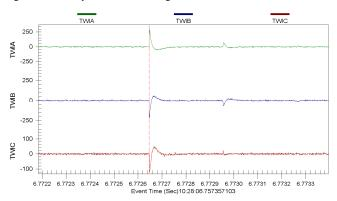
Fig. 16. TWs captured at the receiving end for an AB fault.
