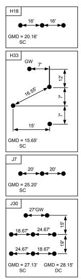
Fig. 20. Tower structures on the Goshen-Drummond line.
