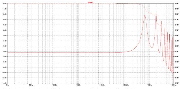
Fig. 9. LTspice simulation showing the peaks in the frequency response caused by the secondary wiring of the CT.
