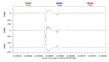
Fig. 24. Phase currents at Goshen for the C-phase-to-ground fault at 67.91 miles from Goshen terminal.
