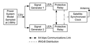
Fig. 12. Test setup using LEA signals to test the TW fault locating system.
