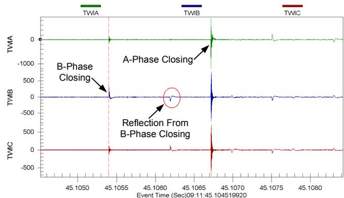
Fig. 23. TW phase currents captured during line energization.
