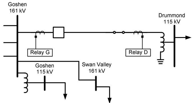
Fig. 21. Transmission network that includes the Goshen-Drummond line.
