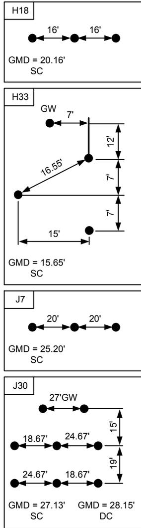
Fig. 20. Tower structures on the Goshen-Drummond line.
