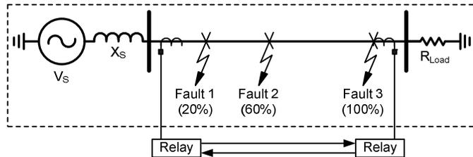
Fig. 17. Physical transmission line model.
