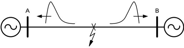
Fig. 3. TWs propagating to Terminals A and B.
