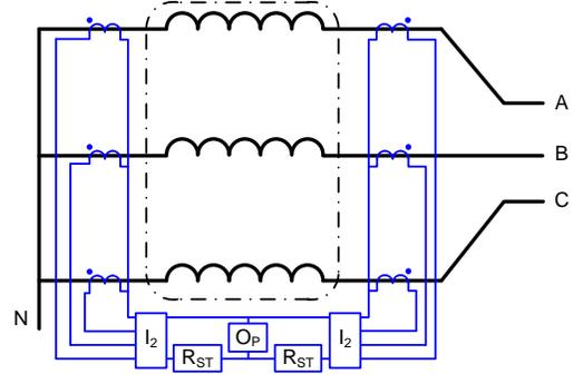
Fig. 13. Negative-sequence differential protection scheme.
