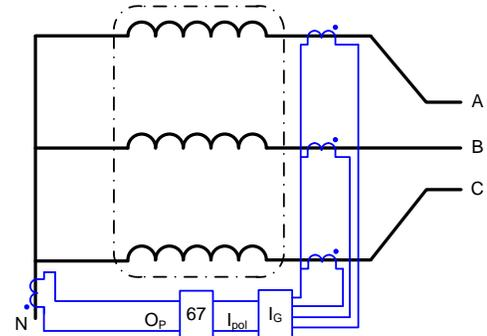
Fig. 14. Restricted earth fault protection scheme.
