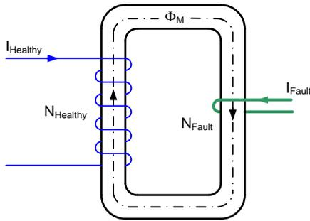
Fig. 7. Two-winding transformer model demonstrates the magnitude in the faulted turn(s) during a turn-to-turn fault.
