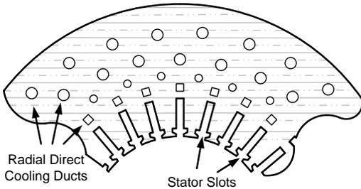
Fig. 1. Laminated stator core showing both the stator slots and the radial cooling ducts used for direct gas cooling.
