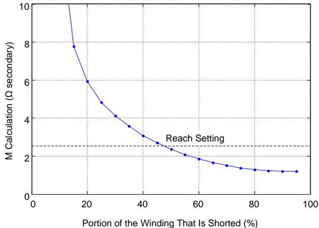
Fig. 19. Impedance versus percent of shorted winding for turn-to-turn faults.
