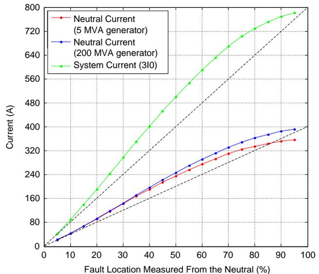
Fig. 18. Ground fault contribution versus location.
