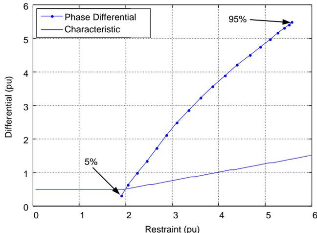
Fig. 17. Phase-to-ground faults plotted on the differential operating characteristic.
