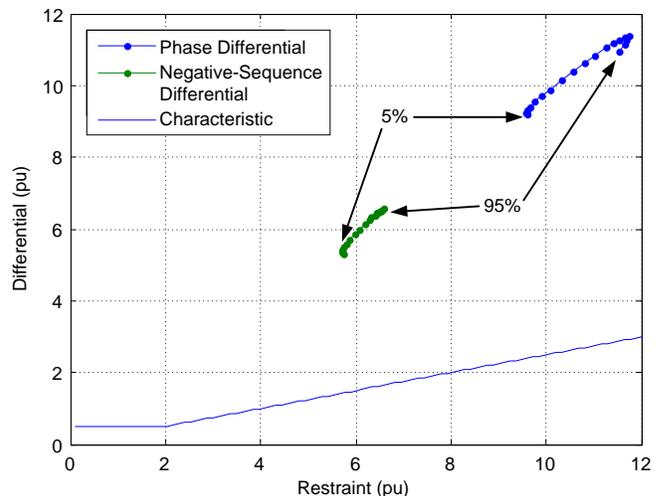
Fig. 16. Phase-to-phase faults plotted on the differential operating characteristic.
