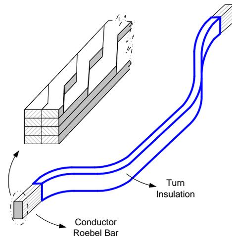
Fig. 4. Sketch of a half-turn coil, or Roebel bar, as would be commonly used in a large (> 50 MVA) generator.
