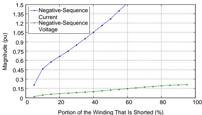
Fig. 21. Negative-sequence current and voltage magnitude versus percent of shorted winding for turn-to-turn faults.
