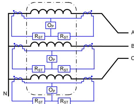
Fig. 11. Biased differential protection scheme.
