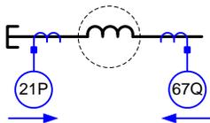
Fig. 20. Turn-to-turn fault protection using a 21P or 67Q element.
