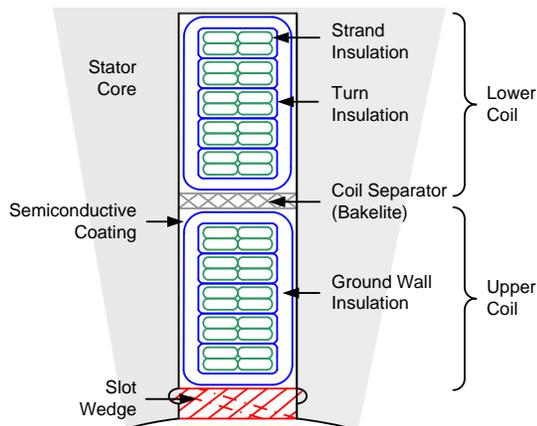
Fig. 6. Sketch of a form-wound stator coil in a double-layer stator winding with four strands and five turns per coil.
