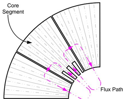
Fig. 2. Stator core segments used to make the stator core of a large diameter hydrogenerator.
