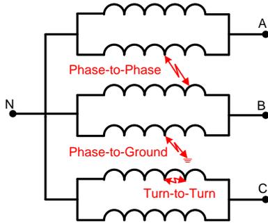
Fig. 9. A sketch showing the different types of faults that can be experienced by a stator winding.
