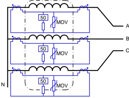
Fig. 12. High-impedance differential protection scheme.
