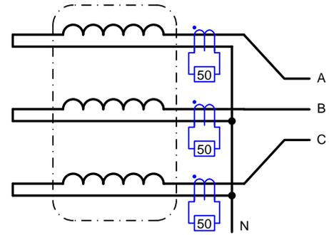
Fig. 10. Self-balancing differential protection scheme.
