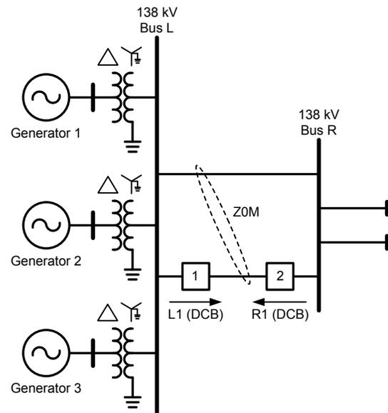
Fig. 1. System one-line diagram.
