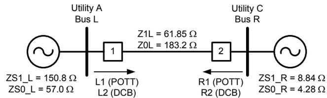
Fig. 16. Protected transmission line for Case 3 (all values are in primary ohms).
