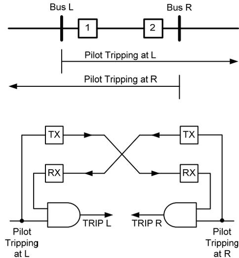
Fig. 4. Permissive overreaching transfer trip logic.
