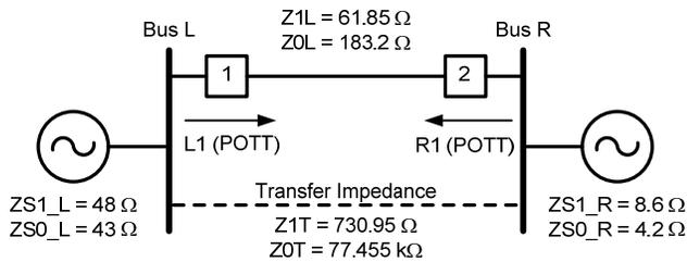
Fig. 8. Simplified equivalent system model (all values are in primary ohms).
