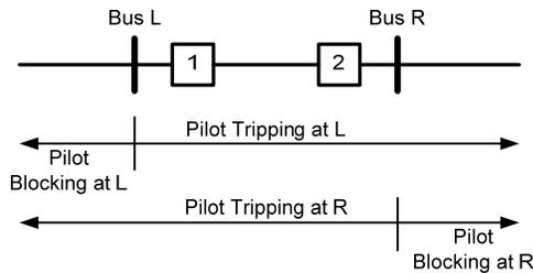
Fig. 5. Relay elements in a hybrid POTT scheme.
