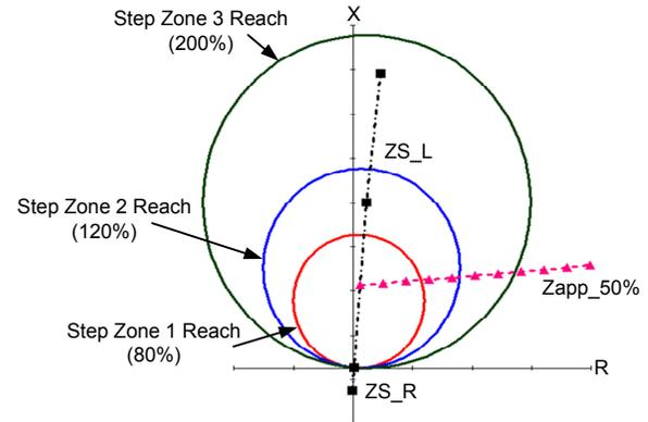
Fig. 10. Mho ground distance elements at Bus R.
