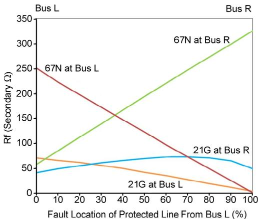
Fig. 13. Fault resistance detection (21G versus 67N elements).
