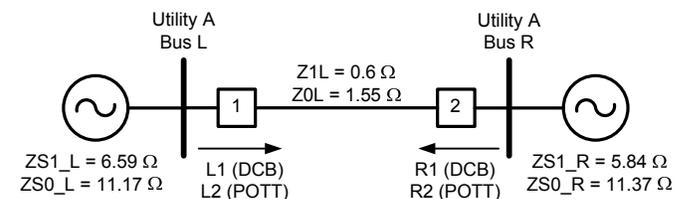
Fig. 14. Protected transmission line for Case 1 (all values are in primary ohms).
