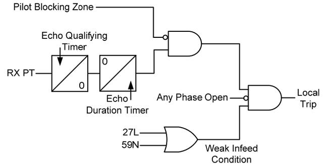
Fig. 7. Weak infeed logic in the hybrid POTT scheme.
