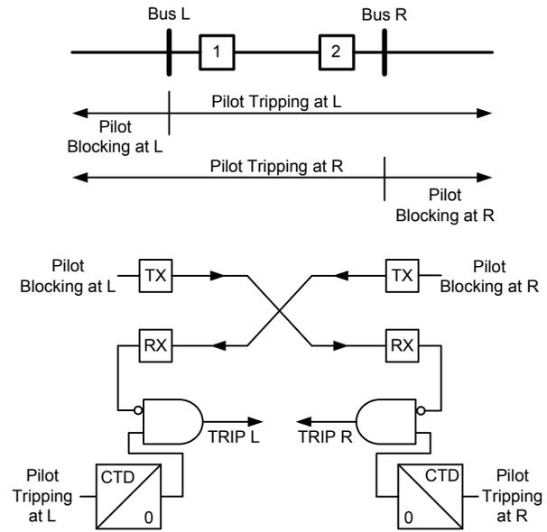
Fig. 2. Directional comparison blocking logic.
