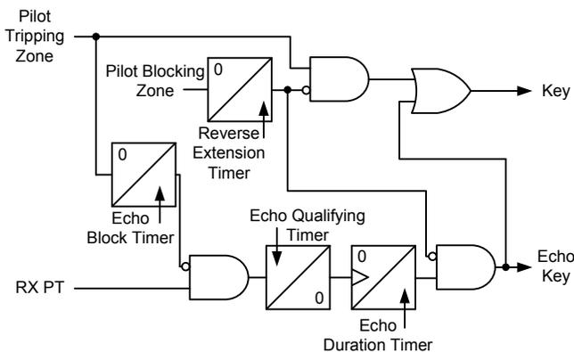
Fig. 6. Echo and current reversal logic in the hybrid POTT scheme.
