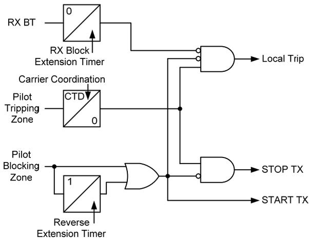
Fig. 3. Advanced DCB logic.
