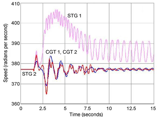
Fig. 4. Generator Speed Plot of 0.28-Second Three-Phase Fault
