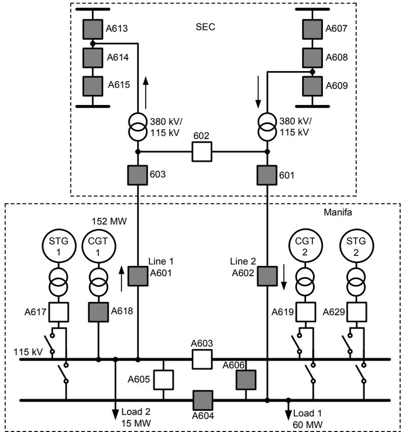
Fig. 13. System Configuration Before Remote-End Trip
