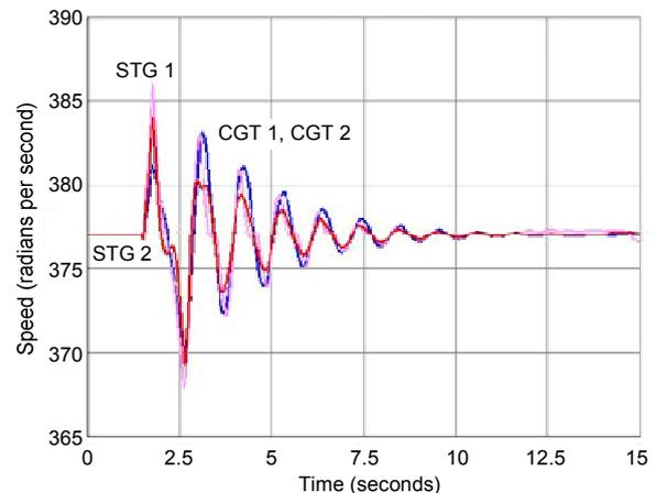
Fig. 5. Generator Speed Plot of 0.27-Second Three-Phase Fault
