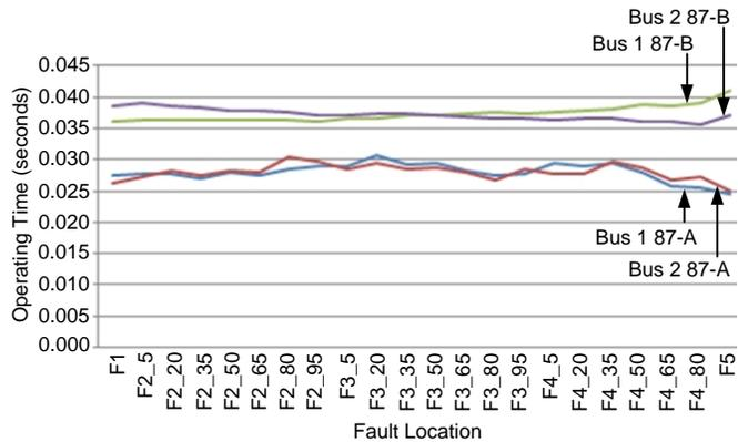
Fig. 9. Sequence differential operating times.
