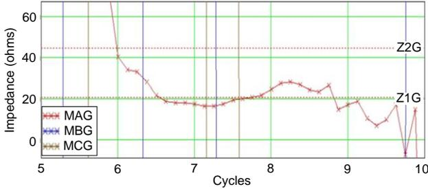
Fig. 6. A-phase ground mho loop calculation.
