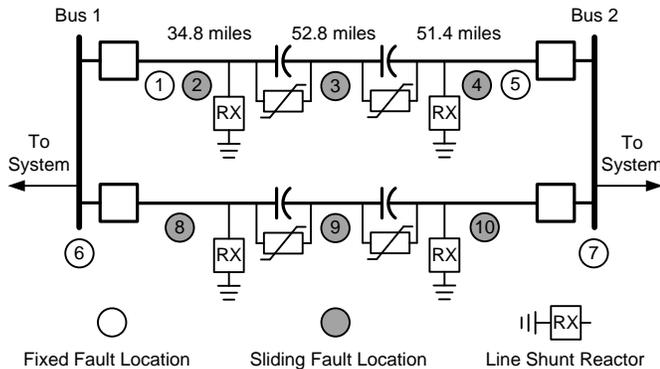
Fig. 5. Reduced system model.
