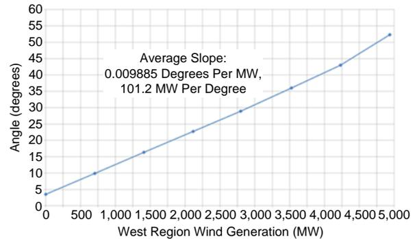
Fig. 2. LCRA line angle study (voltage angle across open Big Hill to Kendall breakers versus west region wind generation).
