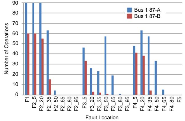
Fig. 7. Zone 1 coverage from Bus 1 87-A and 87-B.
