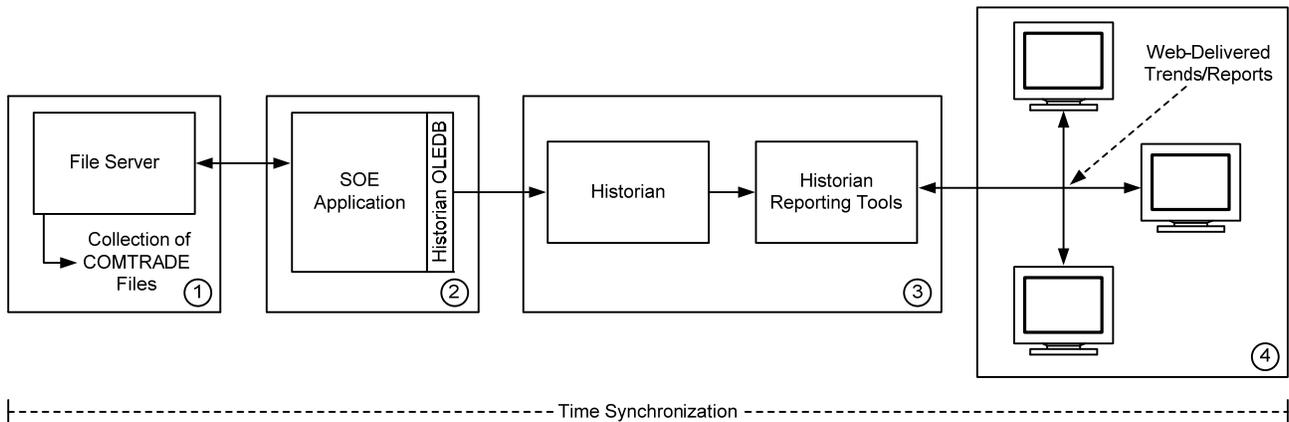
Figure 12. Oscillographic file consumption
