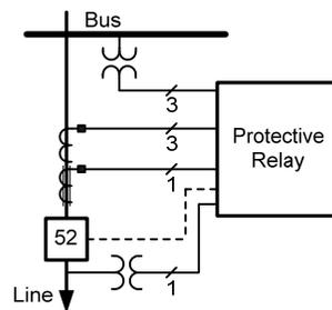
Figure 1. Protection one-line diagram for a feeder relay
