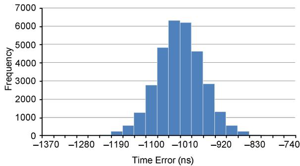
Fig. 12. Time error distribution for connection through a cascade of nontransparent switches (Test 3)
