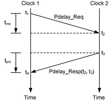
Fig. 5. Synchronization with peer delay mechanism
