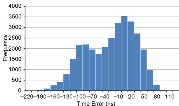
Fig. 20. Time error distribution with a transparent switch and two GOOSE devices (Test 6)
