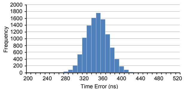
Fig. 9. Time error distributions for connection through a nontransparent switch (Test 2)
