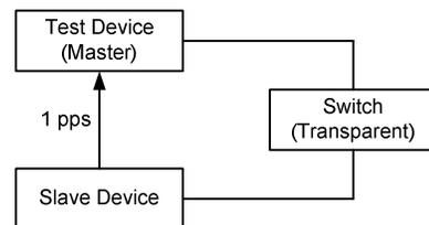
Fig. 16. Test 5: connection through a transparent switch
