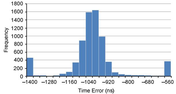
Fig. 14. Time error distribution with a cascade of three nontransparent switches and two GOOSE devices (Test 4)
