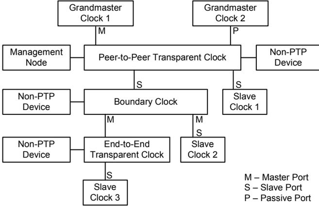
Fig. 3. Example PTP clock hierarchy
