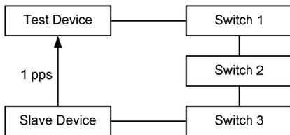
Fig. 11. Test 3: connection through a cascade of nontransparent switches
