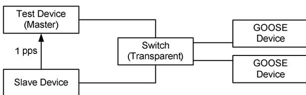
Fig. 19. Test 6: connection through a transparent switch with two GOOSE devices
