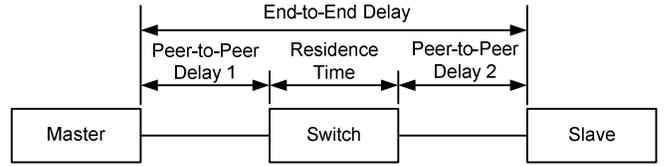
Fig. 1. Relationship between end-to-end and peer-to-peer delay measurements
