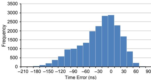
Fig. 18. Time error distribution for connection through a transparent switch with swapped connections (Test 5)
