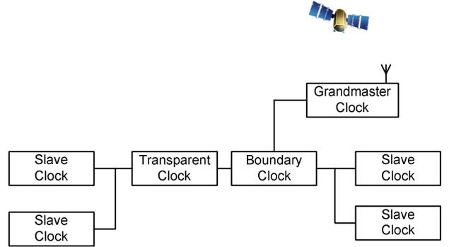
Fig. 2. Example PTP network topology
