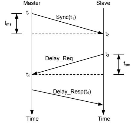
Fig. 4. Synchronization with delay request-response mechanism
