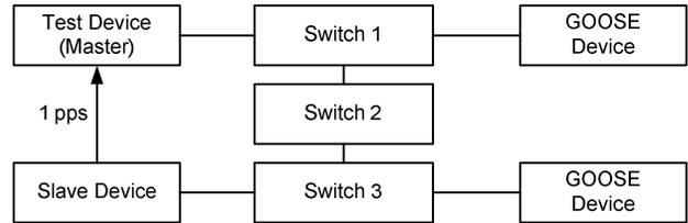
Fig. 13. Test 4: connection through a cascade of nontransparent switches with two GOOSE devices
