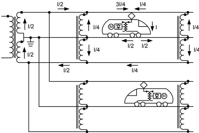
Fig. 3. 2x25 kV Railway System
