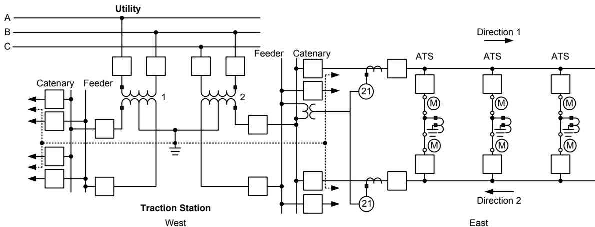
Fig. 17. Parallel Operation of Electrical Railway Feeders
