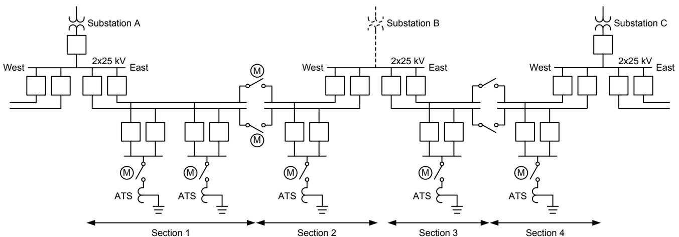
Fig. 5. 2x25 kV and Dual Rail Direction Example
