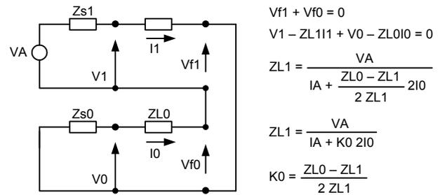
Fig. 12. Phase-to-Ground Fault Loop Impedance
