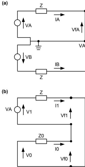
Fig. 10. Phase-to-Ground Fault (a) and Equivalent Sequence Network (b)
