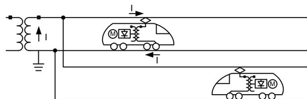
Fig. 2. 1x25 kV Railway System
