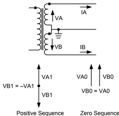
Fig. 8. Symmetrical Components in a Two-Phase System
