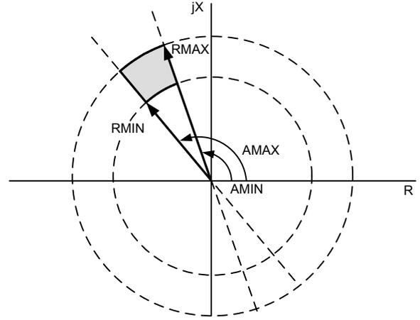
Fig. 22. Wrong Phase Coupling Impedance Area on the ZAB Plane
