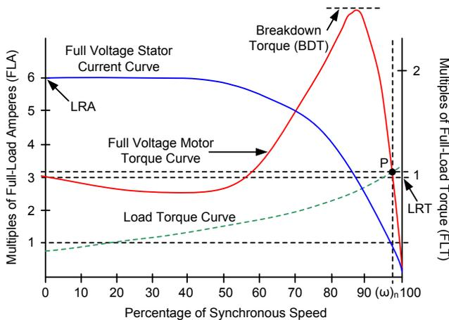
Fig. 1. Typical Motor Operating Characteristics
