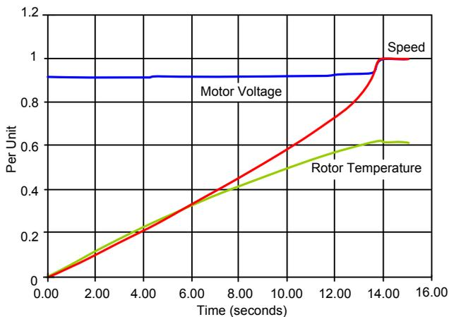
Fig. 12. 27,000 hp Motor Starting Thermal Results
