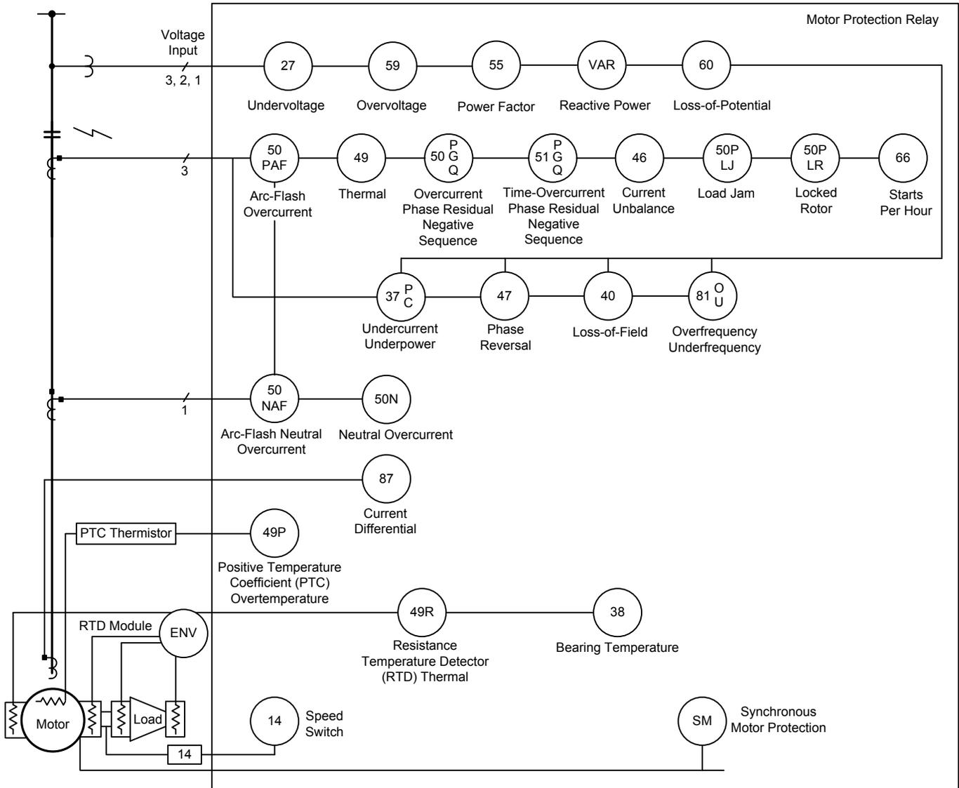
Fig. 2. Standard Features of a Motor Protection Relay
