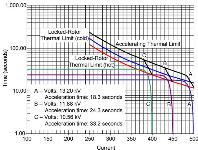
Fig. 7 Locked-Rotor Thermal Limits Versus Current
