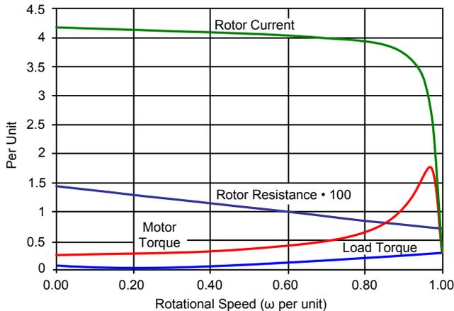
Fig. 5. Motor Starting Current and Torque
