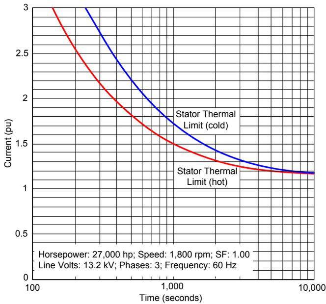
Fig. 6 Stator Thermal Limit Curve for 27,000 hp Motor
