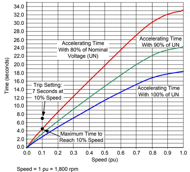
Fig. 8. Starting Time Characteristics Based on Infinite Bus (constant voltage)
