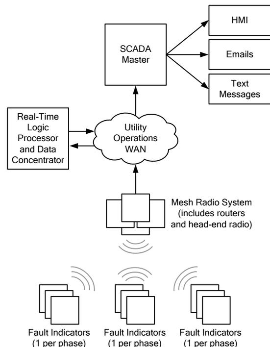
Fig. 1. System diagram showing key components and the communications paths used
