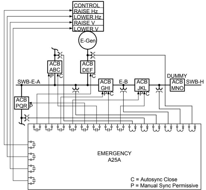
Fig. 3 Platform 1 Emergency Generator A25A
