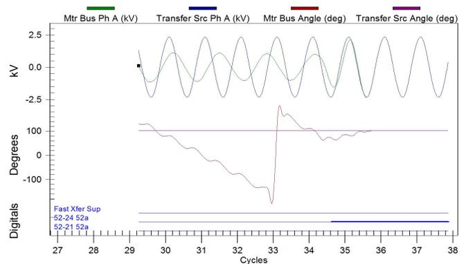
Fig. 12 Relay Test Results for an In-Phase Transfer (Zoomed)
