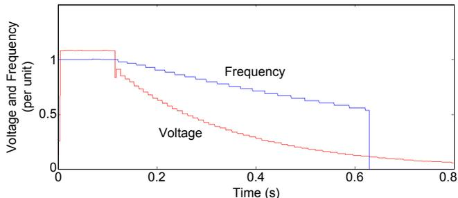
Fig. 1 Rundown Plot of Voltage Magnitude and Frequency Versus Time
