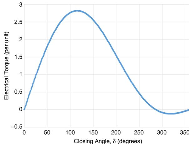
Fig. 3 Electrical Torque Versus Closing Angle in Degrees
