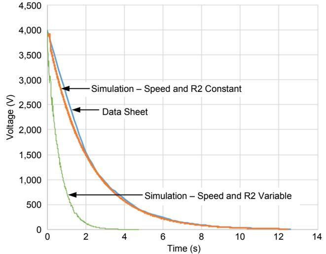
Fig. 6 Voltage Decay Validation
