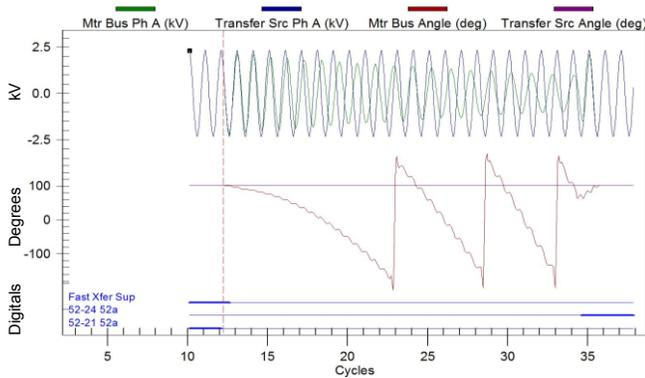
Fig. 9 Relay Test Results for an In-Phase Transfer
