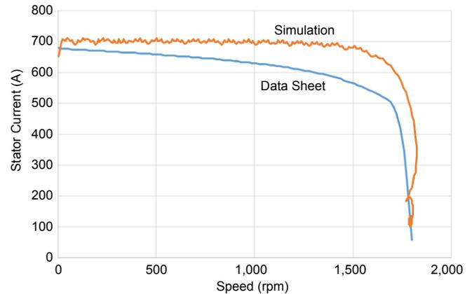
Fig. 8 Motor Starting Current Comparison
