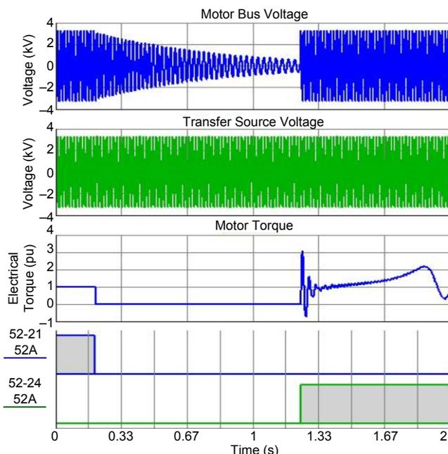
Fig. 13 Simulation Results for a Residual Transfer
