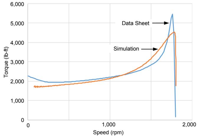
Fig. 7 Motor Torque Comparison
