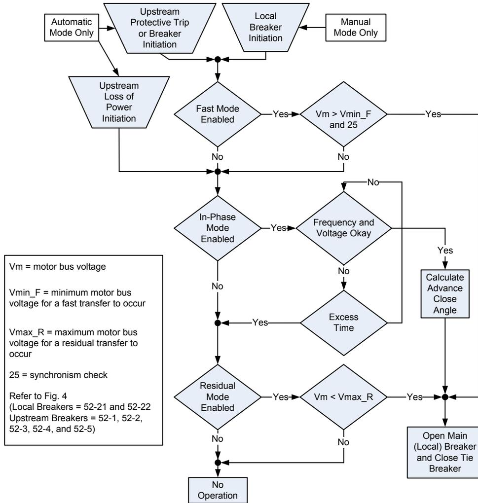
Fig. 5 Motor Bus Transfer Algorithm
