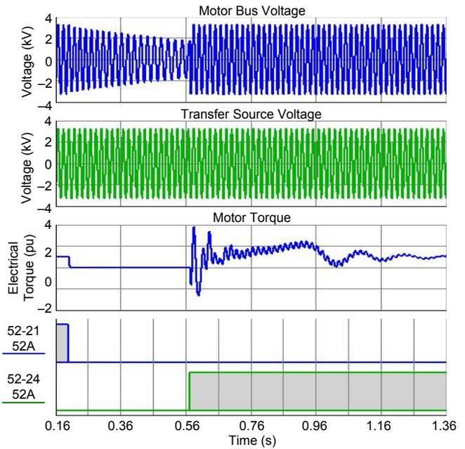
Fig. 11 Simulation Results for an In-Phase Transfer (Zoomed)
