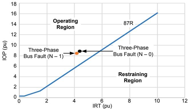
Fig. 9. Substation B bus differential characteristic and simulated internal (bus) faults
