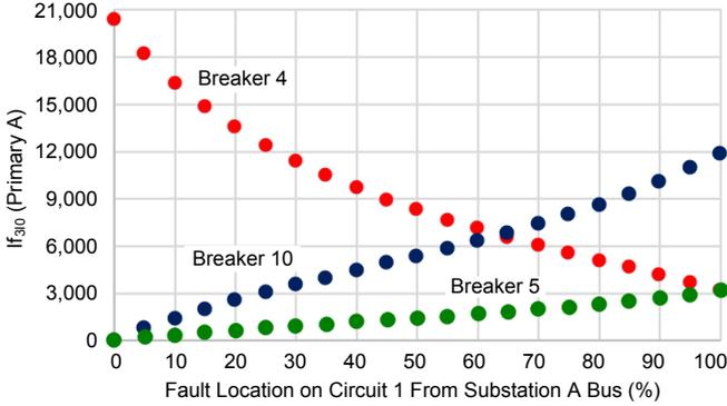
Fig. 3. Fault current variation as seen by Breakers 4, 5, and 10 for faults on Circuit 1
