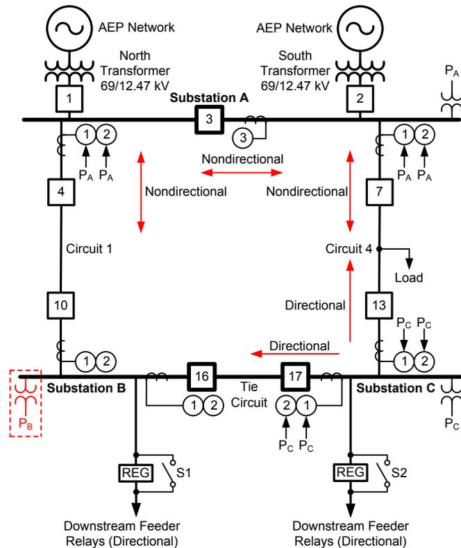
Fig. 14. An LOP condition at Substation B
