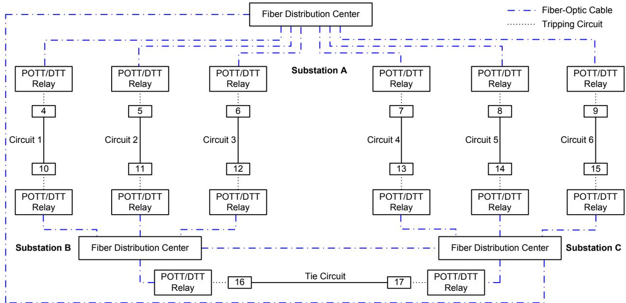
Fig. 11. Network communications layout for the POTT/DTT relay schemes
