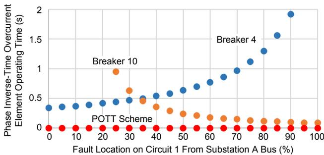
Fig. 12. POTT and phase inverse-time overcurrent element operating times as seen by Breakers 4 and 10 on Circuit 1
