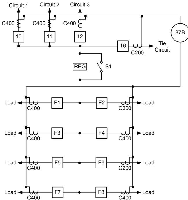
Fig. 6. Existing Substation B bus differential scheme CT connections
