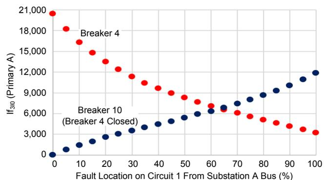
Fig. 2. Fault current variation seen by Breakers 4 and 10 for faults on Circuit 1
