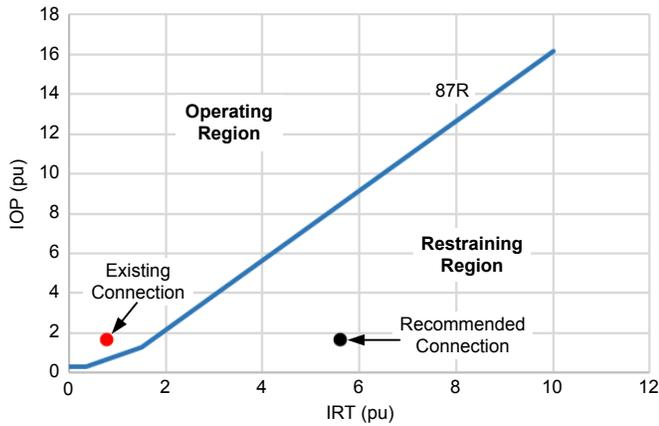
Fig. 8. Substation B bus differential characteristic (recommended versus existing connections)
