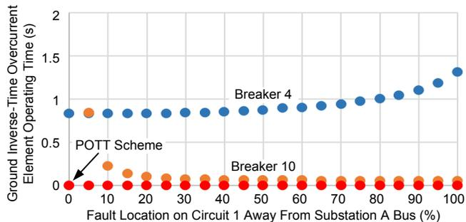
Fig. 13. POTT and ground inverse-time overcurrent element operating times as seen by Breakers 4 and 10 on Circuit 1
