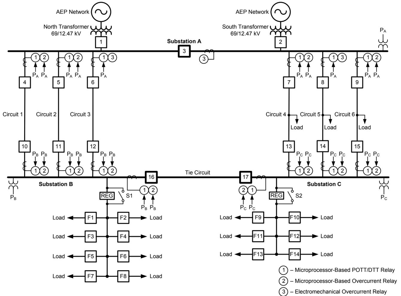
Fig. 1. Simplified one-line diagram of the network
