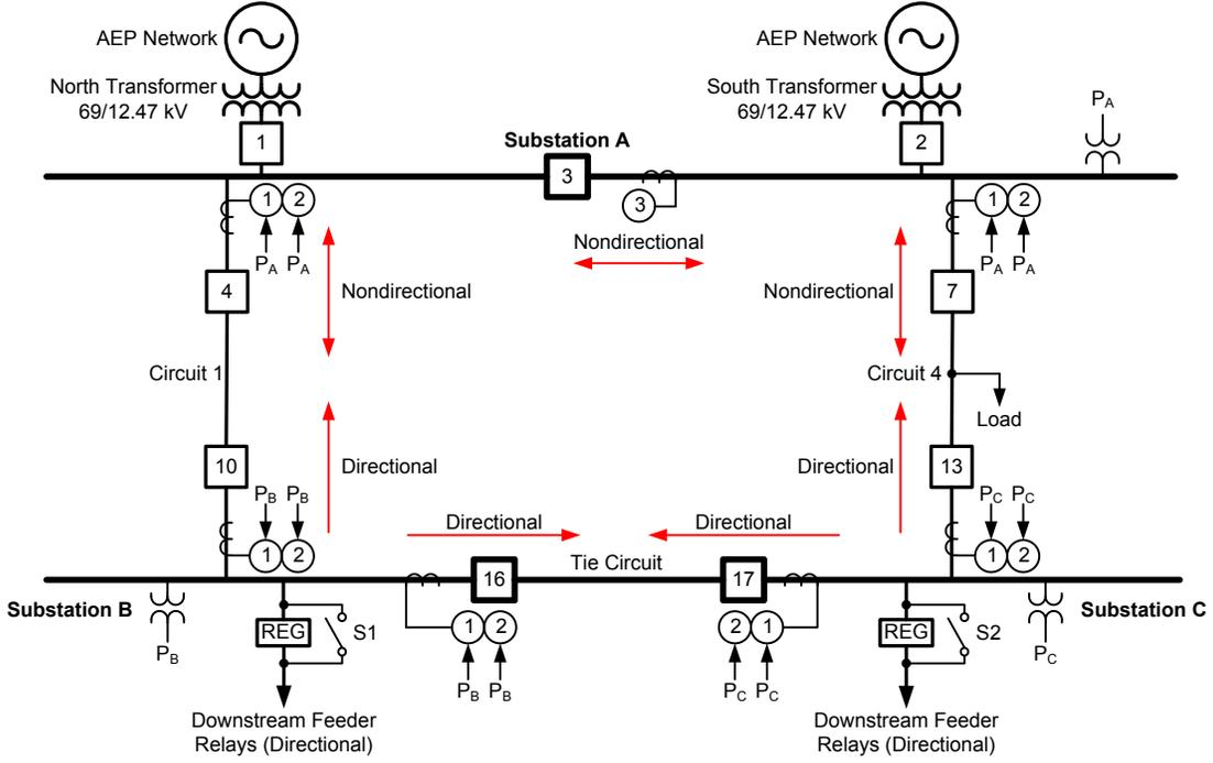
Fig. 5. Simplified one-line diagram showing the use of directional and nondirectional elements
