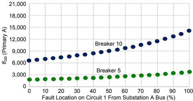
Fig. 4. Fault current variation as seen by Breakers 5 and 10 for faults on Circuit 1 when Breaker 4 is open
