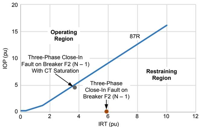
Fig. 10. Substation B bus differential characteristic and simulated external faults
