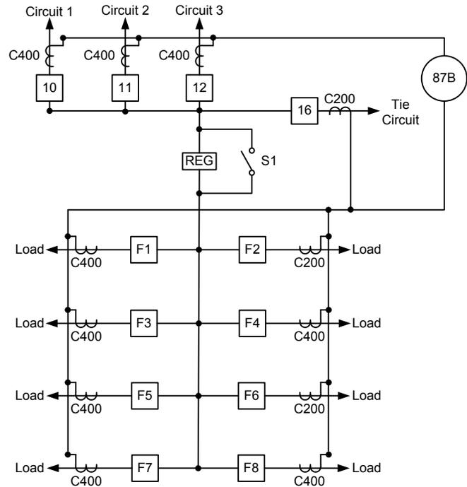
Fig. 7. Recommended Substation B bus differential scheme CT connections
