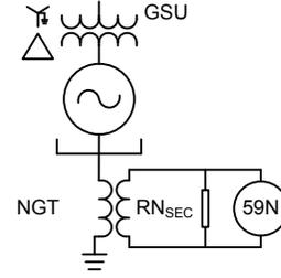
Fig. 6. Generator With Fundamental Neutral Overvoltage (59N) Protection
