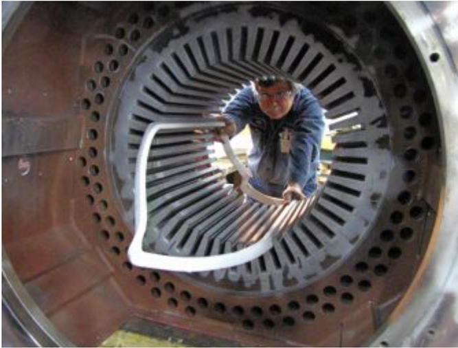
Fig. 4. Insertion of a Form-Wound Coil Winding Into a Small Synchronous Motor
