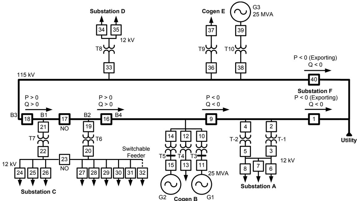
Fig. 1 Simplified One-Line Diagram of the Oil Production Field
