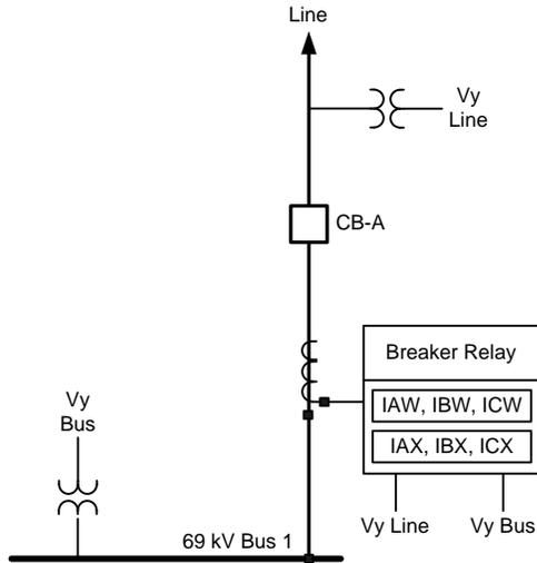
Fig. 2. One-Line Diagram of AEP Breaker Monitoring System
