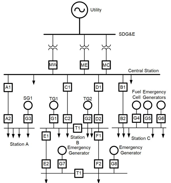
Fig. 1. UC San Diego Simplified One-Line Diagram
