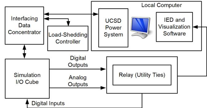
Fig. 11. RTDS Closed-Loop Interface
