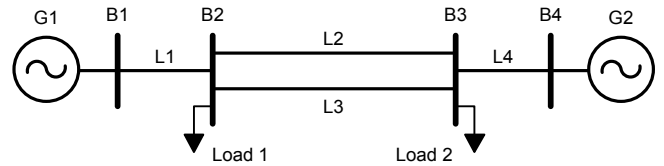
Figure 5. Two-machine test system.
