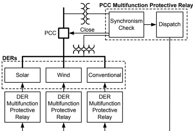
Fig. 2. Multifunction Relays Performing PCC A25A Function
