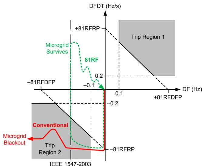
Fig. 6. 81RF Element Assists Microgrid Survival
