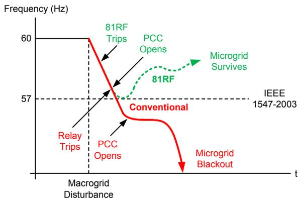
Fig. 7. Proactive Automatic Islanding Before a Microgrid Blackout
