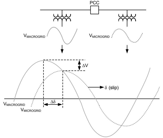
Fig. 3. Relay Performing Synchronism Check
