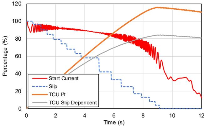
Fig. 9. Slip-Dependent vs  $I^2t$  Thermal Model
