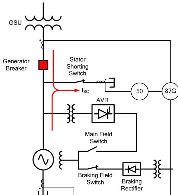
Fig. 18. Dynamic Braking Overcurrent Protection
