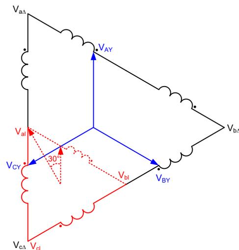
Fig. 12. Reduced-Voltage Starting Using Two Midwinding Taps
