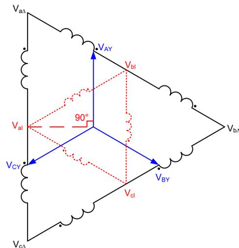
Fig. 11. Reduced-Voltage Starting Using Three Midwinding Taps
