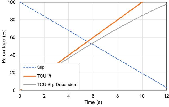
Fig. 8. Slip-Dependent vs  $I^2t$  Thermal Model Assuming Constant Current Magnitude
