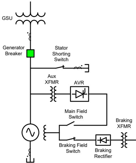
Fig. 15. Typical Configuration of a Dynamic Braking Setup for a Reversible PSH Unit
