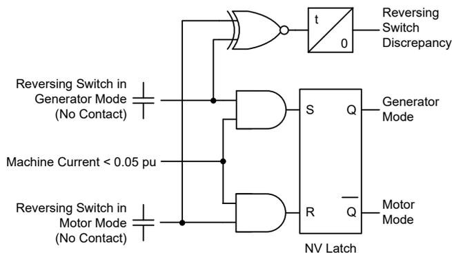
Fig. 7. Operating Mode Logic
