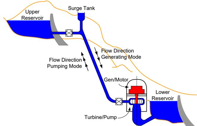
Fig. 1. Pumped Storage Hydro Scheme
