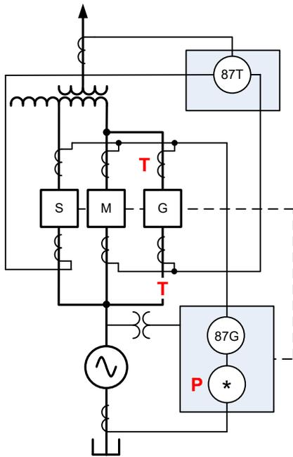
Fig. 13. Reduced-Voltage Starting With Individual Breakers
