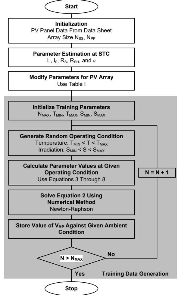
Fig. 3. Proposed method to generate input-output data set for ANFIS training
