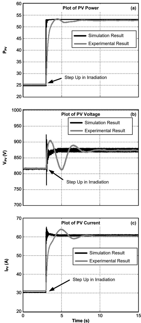
Fig. 10. Comparison of experimental and simulation results of solar park power output (a), voltage (b), and current (c)
