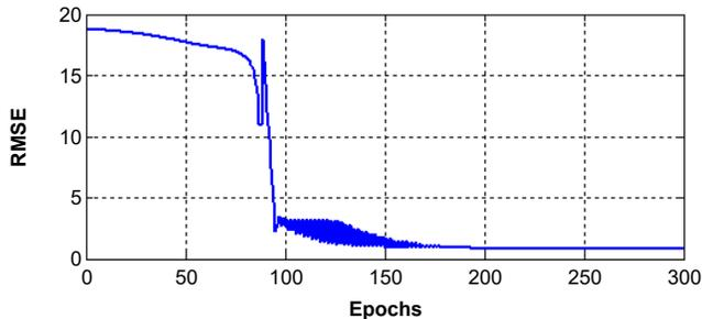
Fig. 6. RMSE versus epochs for the ANFIS-based MPPT controller
