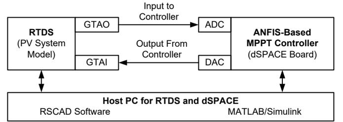
Fig. 5. Hardware-in-the-loop block diagram
