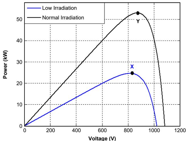
Fig. 7. PV curve under normal and low irradiation
