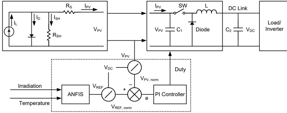
Fig. 4. PV system equipped with the proposed ANFIS-based controller
