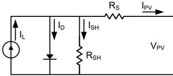
Fig. 1. Equivalent electric circuit of a PV device
