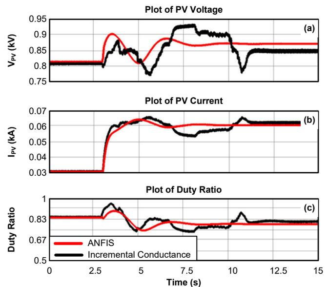
Fig. 9. PV solar park voltage (a), current (b), and duty cycle (c)
