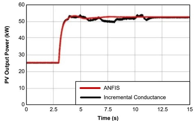
Fig. 8. PV solar park output power
