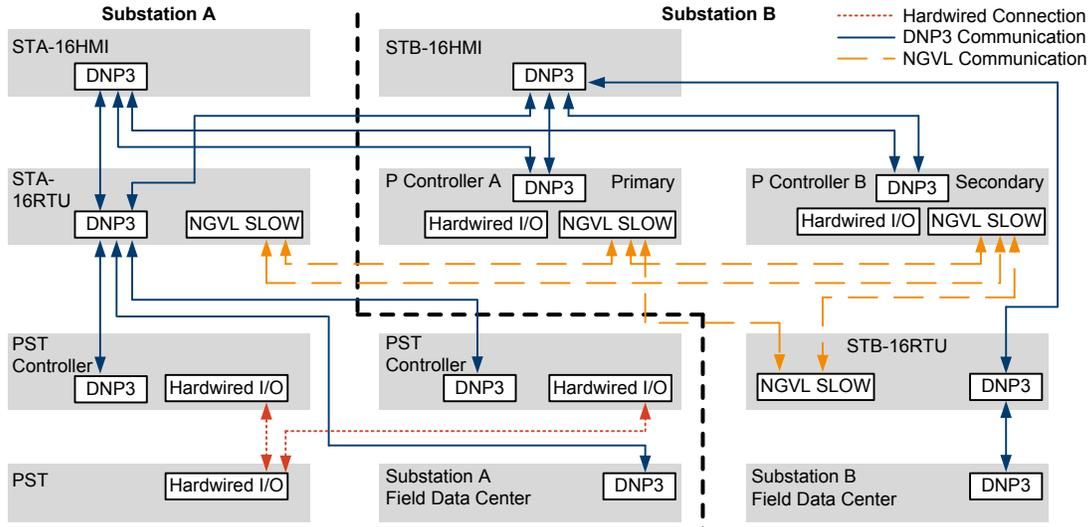
Figure 1. Data Flow Diagram (DFD) of P Control System
