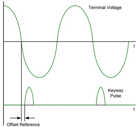
Fig. 7. Rotor and Voltage Physical Relationship
