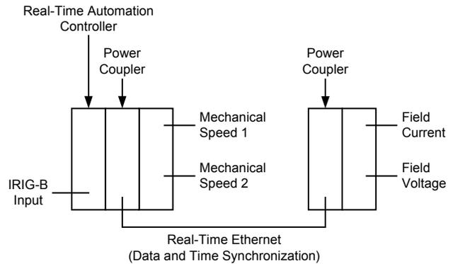
Fig. 9. Generator Monitoring System Architecture
