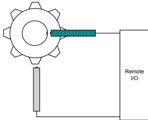
Fig. 8. Toothed Wheel Data Acquisition
