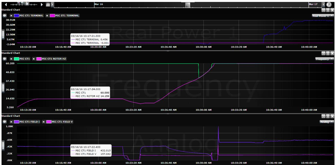
Fig. 15. Starting Curve for LCI Start
