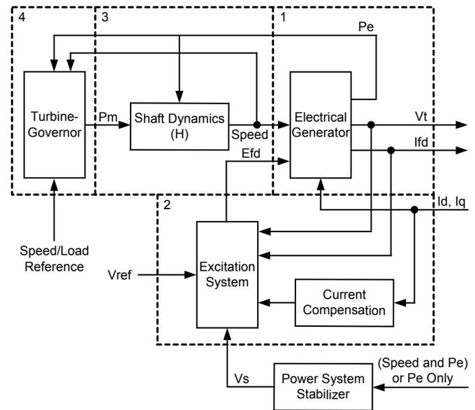
Fig. 2. Typical Generator Plant Subsystems [4]
