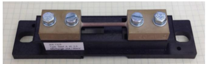
Fig. 5. Shunt Resistor
