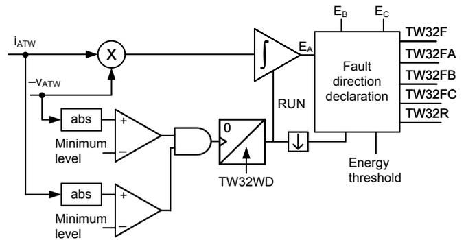
Fig. 2. Simplified logic of the TW32 element.
