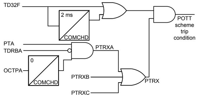
Fig. 4. Receiver logic provides security to the POTT scheme.
