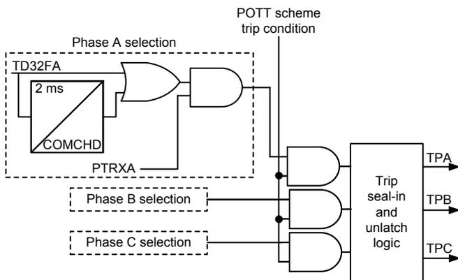
Fig. 5. Phase selection and trip logic for the POTT scheme.
