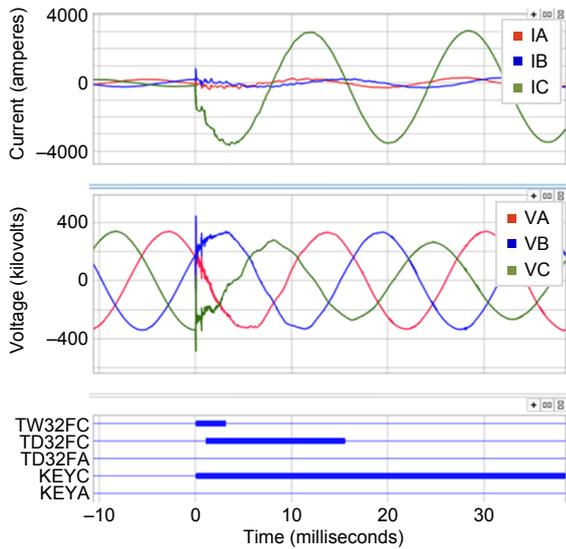
Fig. 6. Currents and voltages captured at MID and the time-domain protection element operation for the internal fault on May 4.
