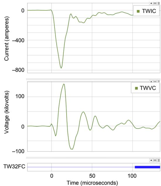
Fig. 8. TW current and voltage captured at MID and the TW32 protection element operation for the internal fault on May 4.
