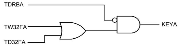
Fig. 3. Key transmitter logic for accelerating the POTT scheme.
