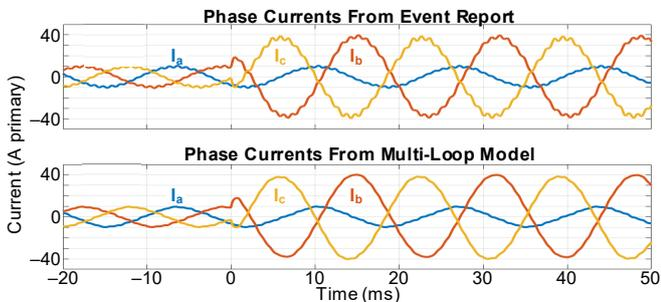
Fig. 2. Response comparison between the scale-model machine (top) and the simulation (bottom) for an external phase-to-phase fault.
