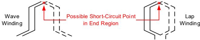
Fig. 4. Possible fault points in the end-winding region for wave and lap winding configurations.
