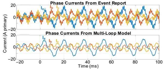
Fig. 3. Response comparison between the scale-model machine (top) and the simulation (bottom) for a five-turn interturn fault.
