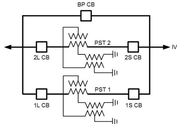
Fig. 1. Two-Core PST – Simplified One-Line Diagram
