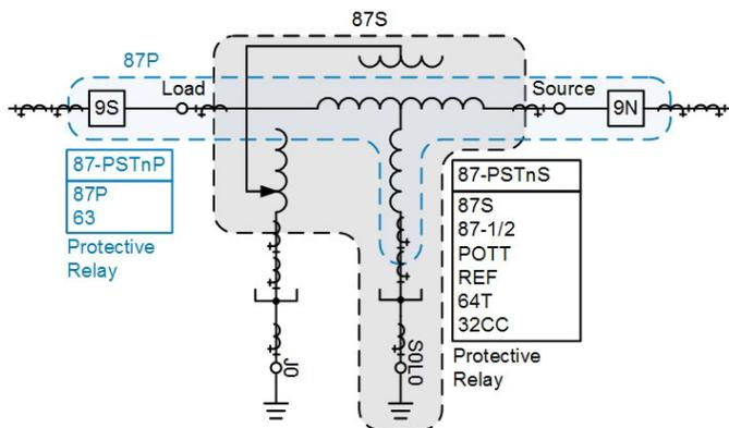
Fig. 5. Main 1 Primary and Secondary Protection
