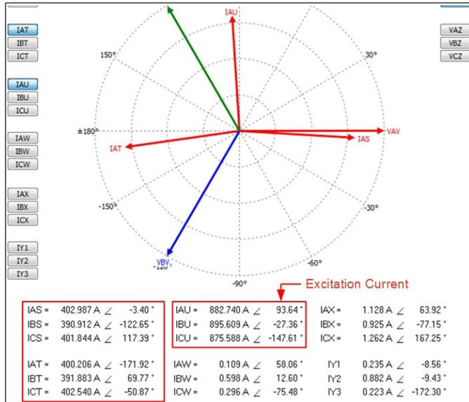
Fig. 21. 160 MW, 87S and 87O Relays Phasors Uncompensated
