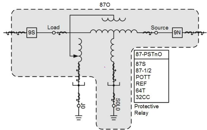
Fig. 6. Main 2 Overall Differential Protection
