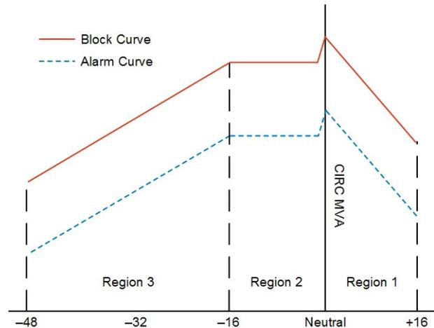
Fig. 13. Circulating MVA Operating Curves
