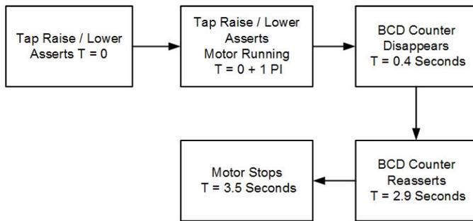
Fig. 18. PST Typical Tap-Change Operation Timing Diagram
