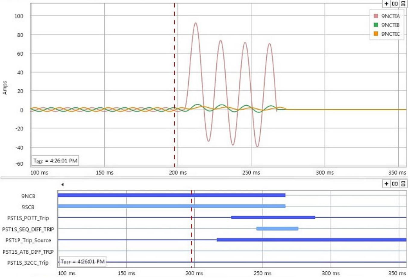
Fig. 16. Single-Phase Internal Fault at FLOC 1 Tap Neutral
