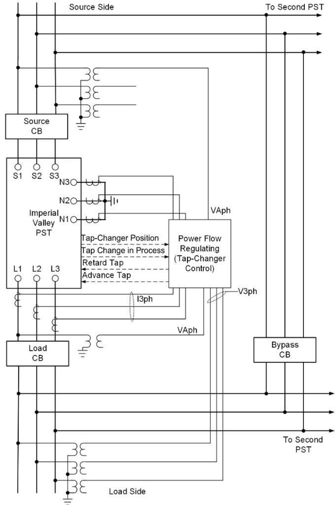
Fig. 11. PST Connection Diagram
