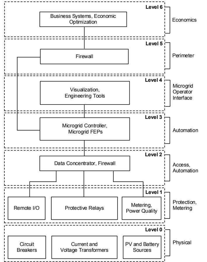
Fig. 3. Segmented MGCS architecture
