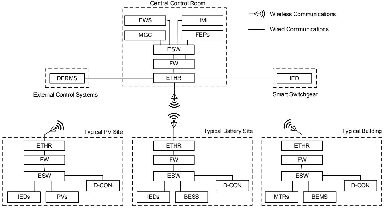
Fig. 4. Overall MGCS network architecture
