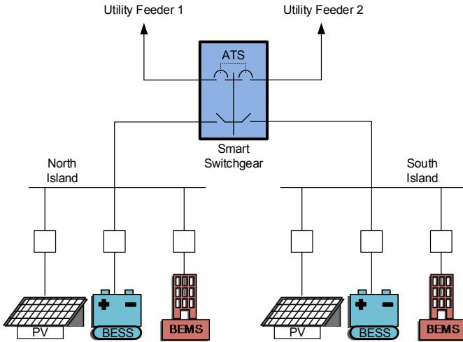
Fig. 2. Simplified one-line diagram of proposed microgrid
