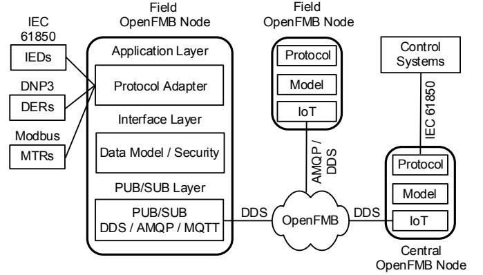
Fig. 6. Example OpenFMB framework model
