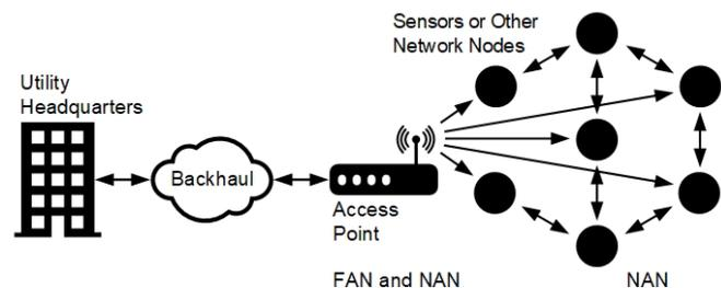
Fig. 2. Wi-SUN System Architecture
