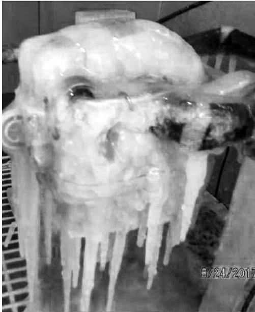
Fig. 6. Ice Buildup Test on Wireless FCI
