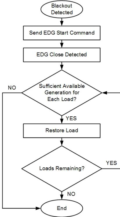
Fig. 10. EBS System Logic Flow
