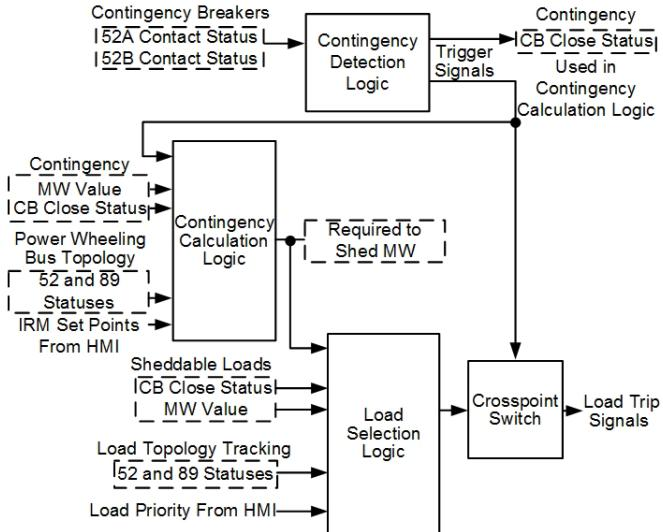
Fig. 7. CLS System Algorithm
