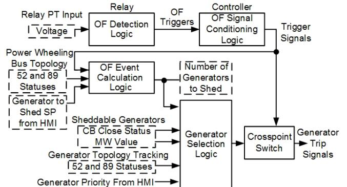
Fig. 9. OFGS System Algorithm
