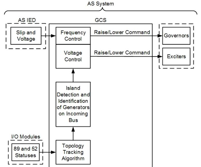
Fig. 6. Autosynchronization Control System
