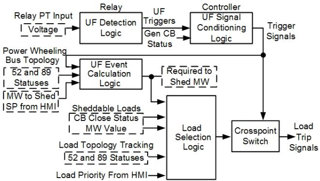
Fig. 8. UFLS System Algorithm
