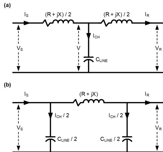
Fig. 1. (a) T-Model of a Transmission Line; (b)  $\pi$ -Model of a Transmission Line
