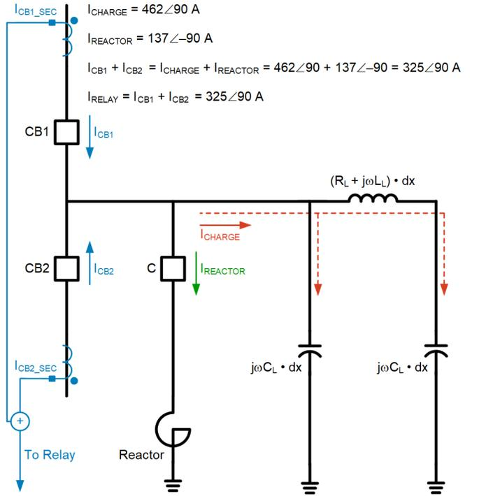
Fig. 5. Reactor Current Included in Differential Protection Zone
