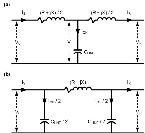
Fig. 1. (a) T-Model of a Transmission Line; (b)  $\pi$ -Model of a Transmission Line
