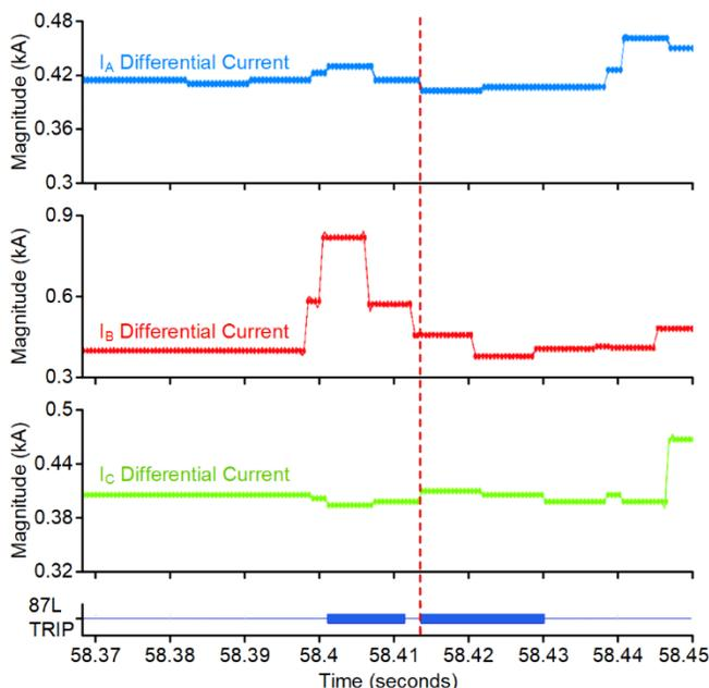
Fig. 4. Differential Current Event Record From Station A 87L Relay
