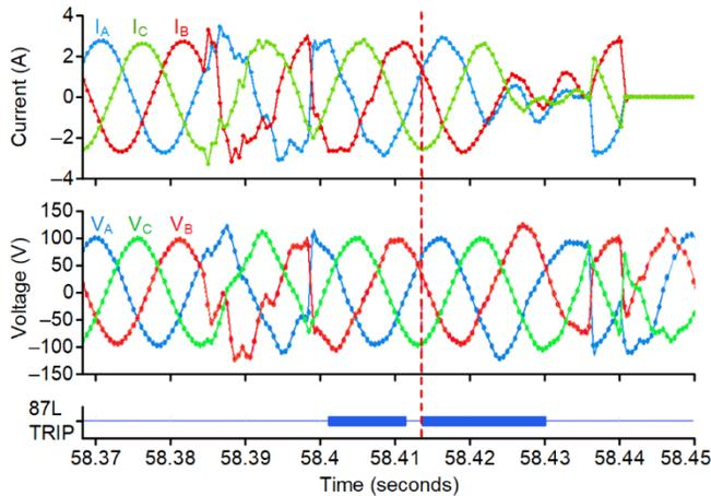
Fig. 3. Current and Voltage Event Record From Station A 87L Relay
