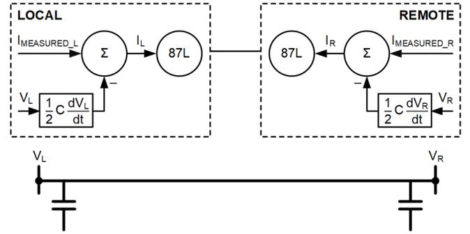
Fig. 2. Subtracting Line Charging Current From the 87L Scheme
