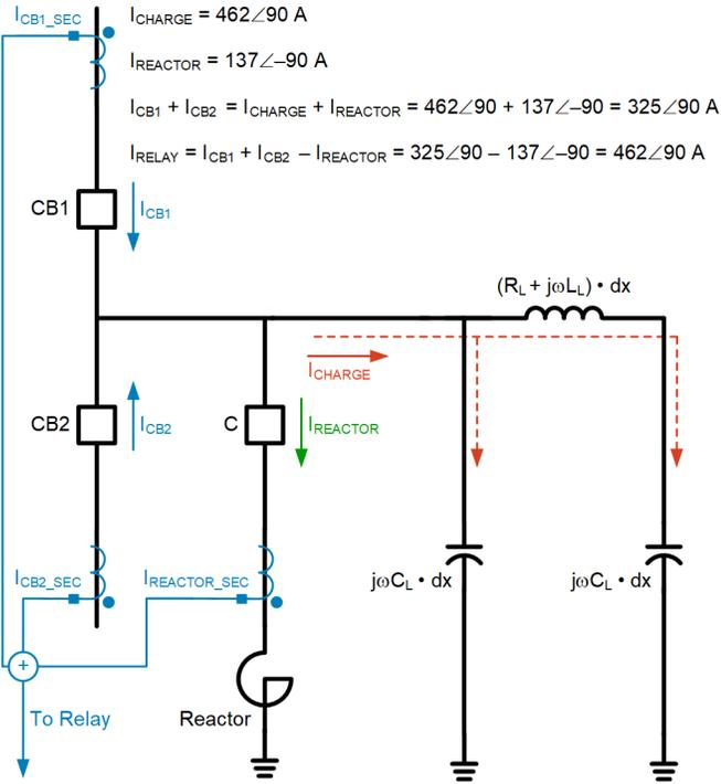
Fig. 6. Reactor Current Excluded From Differential Protection Zone
