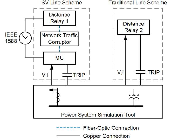
Fig. 17. Test setup with network traffic corruptor
