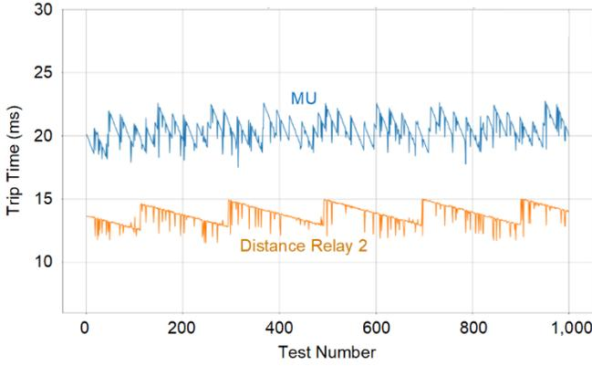
Fig. 16. Benchmark test results (performance comparison of SV distance scheme versus traditional distance relay)
