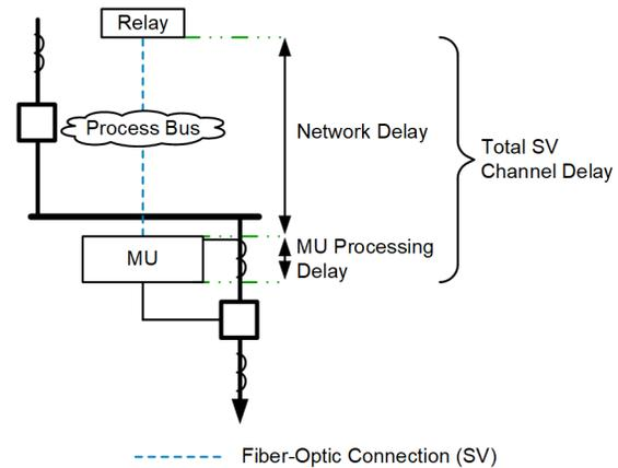
Fig. 3. Network delay and MU processing delay
