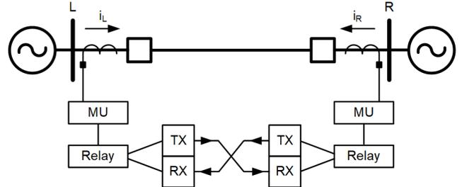
Fig. 6. Line differential protection scheme with two terminals in SV-based substations
