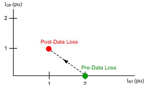
Fig. 9. Effect of losing SV data in a percentage differential application
