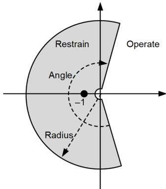
Fig. 8. Traditional Alpha Plane operating characteristic
