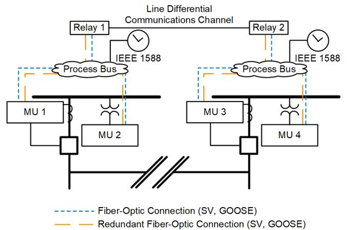
Fig. 2. Line differential protection scheme with a process bus network
