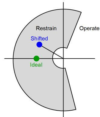
Fig. 12. Effect of uncompensated data acquisition delay mismatch on the Alpha Plane during normal load
