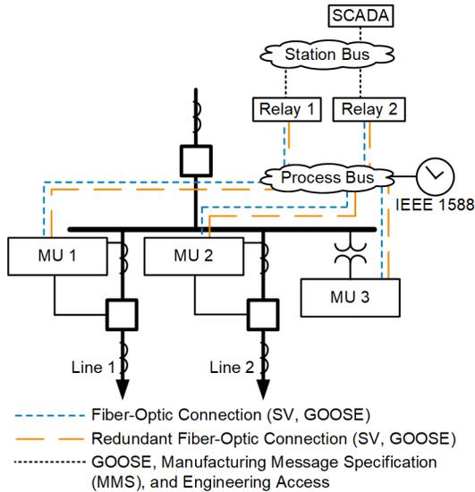
Fig. 1. Line distance protection scheme with a process bus network
