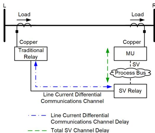
Fig. 11. Hybrid line differential installation with a traditional relay and an SV relay
