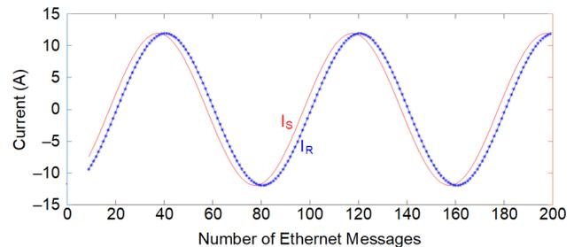
Fig. 4. Example of phase difference introduced by an uncompensated signal
