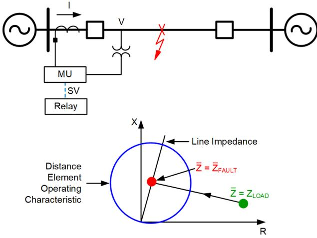
Fig. 13. Impedance plane representation of distance element operation
