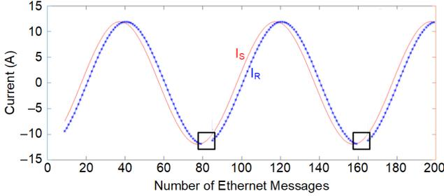
Fig. 5. Example of packet loss in addition to a phase difference introduced by an uncompensated signal
