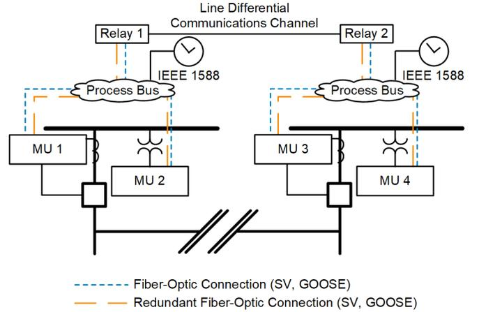
Fig. 2. Line differential protection scheme with a process bus network
