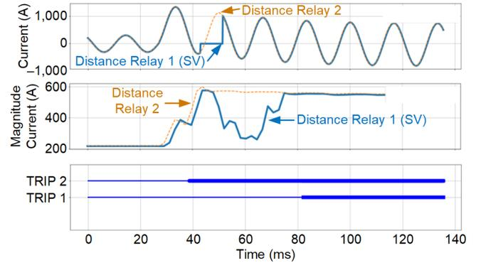
Fig. 18. Packet loss results
