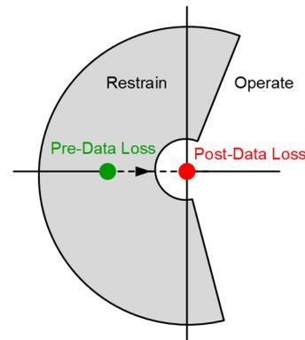
Fig. 10. Effect of losing SV data in an Alpha Plane line differential application
