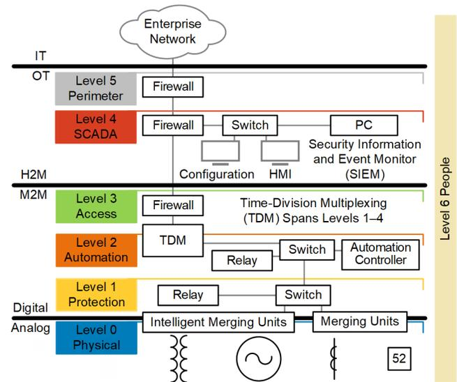
Fig. 2. Defense-in-Depth Levels Diagram
