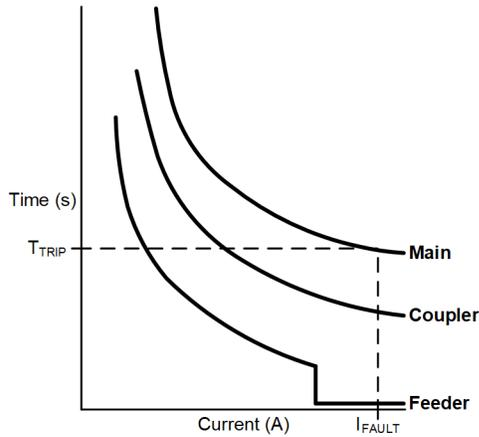
Fig. 2. Long Tripping Time for Bus Section Fault
