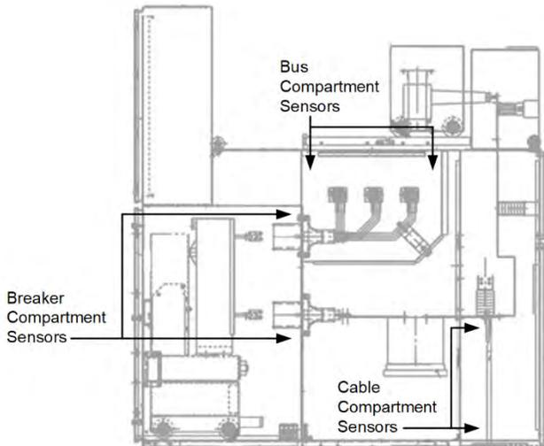
Fig. 9. Arc-Flash Detection Sensor Arrangement in Switchgear Panel
