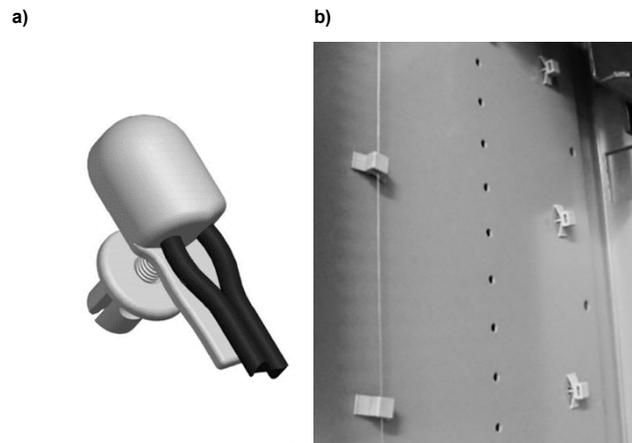
Fig. 7. Light Sensor Types Include a) Point Sensors and b) Bare-Fiber Sensors
