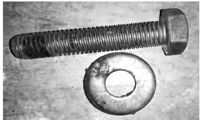
Fig. 19. Stray Bolt and Washer Found Near Fault Location
