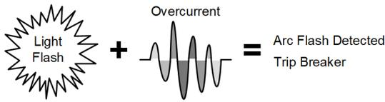
Fig. 5. Simple Combined Tripping Requirements in an Arc-Flash Protection Scheme
