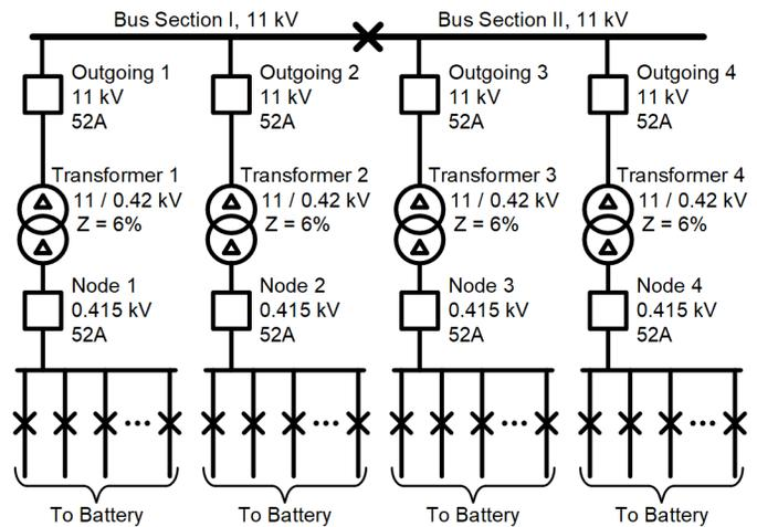
Fig. 8. One-Line Diagram of the 11/0.420 kV Switchboard
