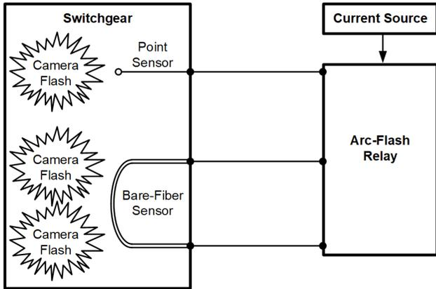
Fig. 15. Testing Configuration for Arc-Flash Detection System
