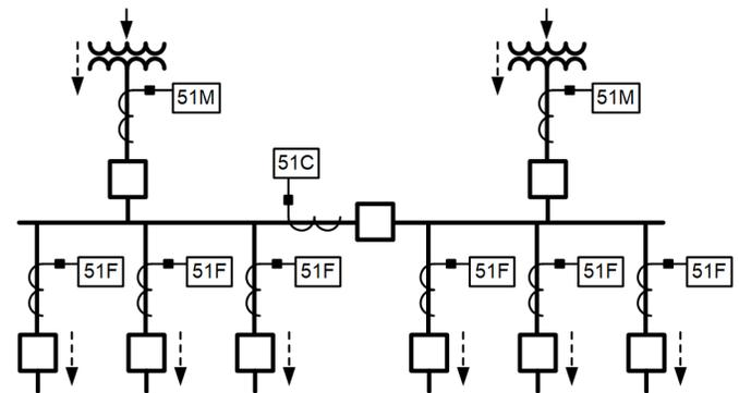
Fig. 1. Typical Double-Bus Configuration for Medium- and Low-Voltage Installations
