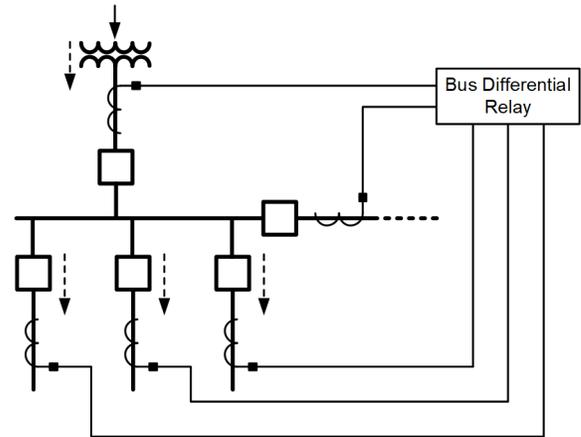
Fig. 4. Bus Differential Protection Scheme Connection Setup
