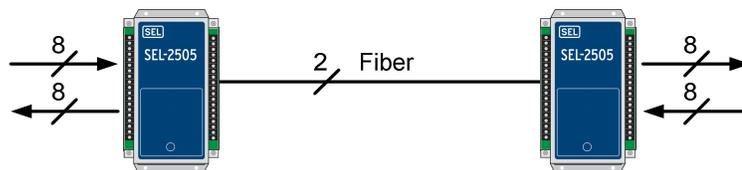
**Figure 1 Eight Inputs Drive Eight Outputs Bidirectionally Over a Fiber Pair**
