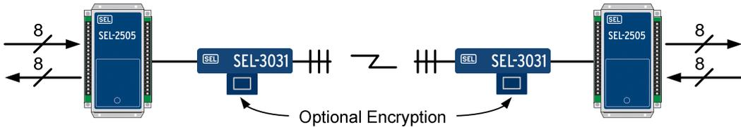
Figure 4 I/O Communications Using an Unlicensed Radio Link
