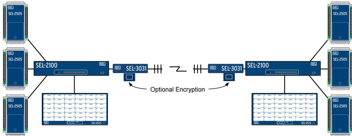
**Figure 8 Mirrored Alarming at Remote Locations Provides Critical Information at Multiple Sites**
