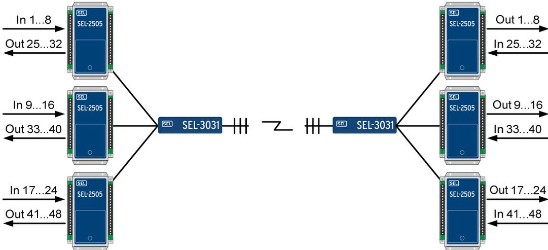
Figure 5 Three Serial Links of Information Can Transmit on a Single Radio
