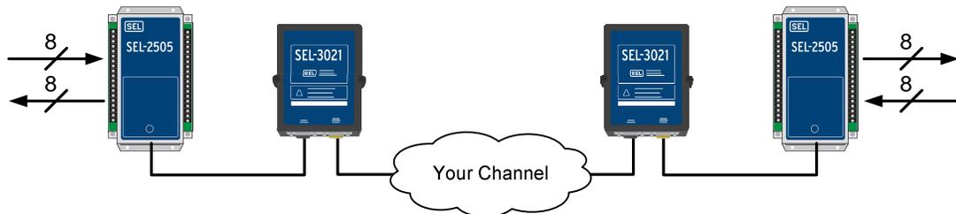
**Figure 3 I/O Communications Including Secure Signal Encryption**
