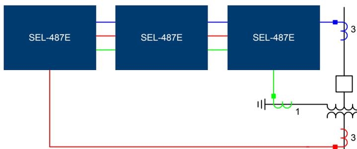
**Figure 2 Proposed GSU Transformer Protection One-Line Diagram**
