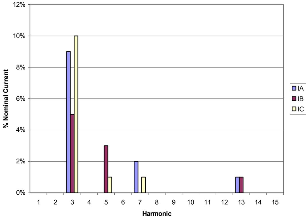
**Figure 4: Harmonics in the Manufacturing Building Power System**
