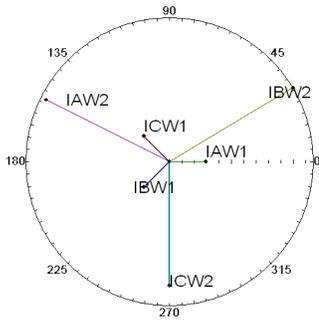
Fig. 14. Winding Currents (7 – Transformer Commissioning Settings 587.pdf)
