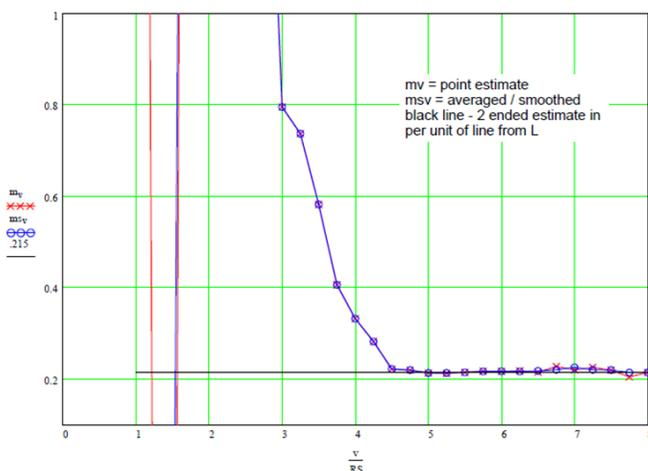
The two-ended result puts the fault at 0.215 per unit of the line from the left, or at 17.6 miles from Substation R. This precisely matches the physical evidence reported by the customer.
