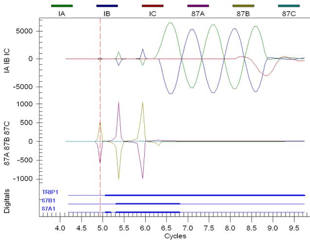
Fig. 24. Raw Bus Differential Operation (11 – High Impedance Bus Trip 587Z Raw.cev)
