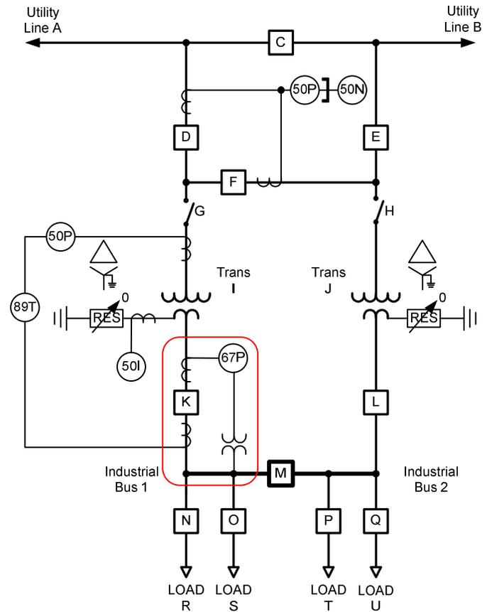
Fig. 5. One-Line Diagram for Directional Element Operation
