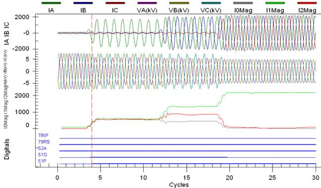
Fig. 2. Distribution Feeder Fault (2 – Distribution Feeder Fault 351A.cev)
