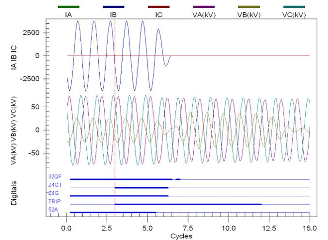
Fig. 21. Third Event, Terminal B (9 – B Delayed Fault Clearing 3rd Event 311C.cev)
