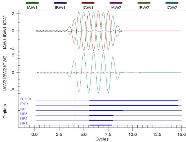
Fig. 8. Phase Currents (5 – Transformer Filtered Event 387A.cev)
