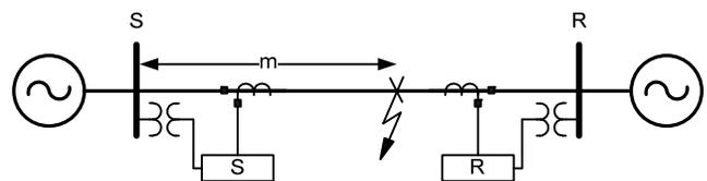
Fig. 9. Fault location on a two-source power system
