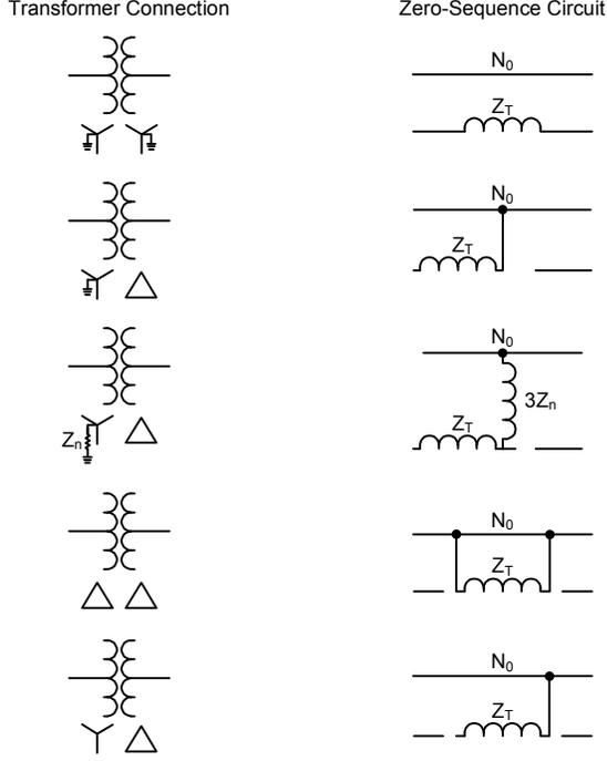
Fig. 1. Zero-sequence circuits for various transformer types
