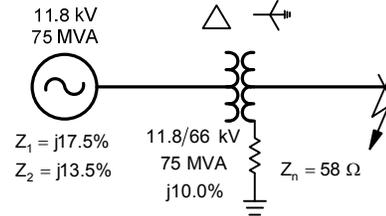
Fig. 7. One-line diagram for fault current calculations
