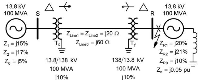
Fig. 8. One-line diagram of a nonradial system
